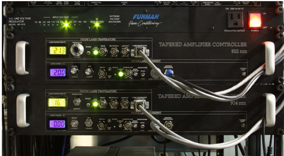
Fig. 12. Photograph of front panels of complete systems for current and temperature control of two TAs.<sup>36</sup>
