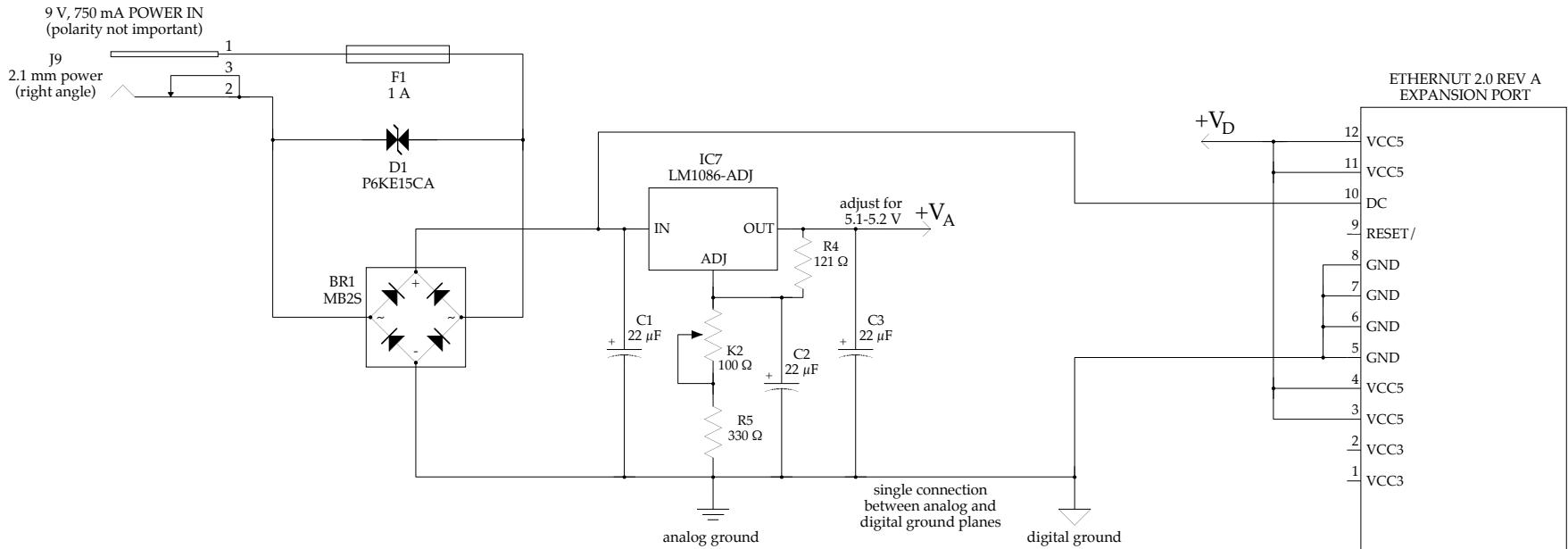
POWER SUPPLY AND REFERENCE BYPASSING (IC1-IC4)
