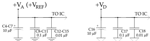
POWER SUPPLY BYPASSING (IC6)
